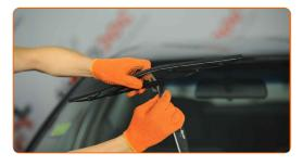
Remove the blade from the wiper arm.
