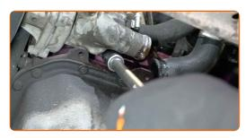
Remove the thermostat housing.
