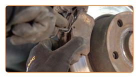
11 Remove the brake disc.
