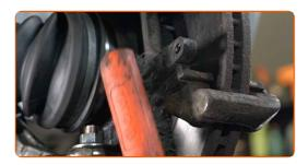
Unscrew the caliper bracket fastening. Use a drive socket #17. Use a tap wrench. Use a ratchet wrench.
