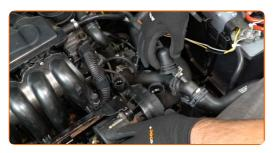
Cover the secondary air pump channels with a microfibre cloth to prevent dust and dirt from getting inside.
