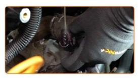
Treat the spark plug wire connectors. Use electronic spray.
