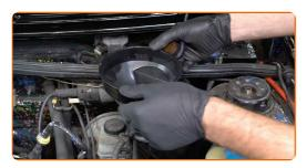
Pour coolant in the coolant reservoir.
