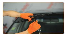
Remove the blade from the wiper arm.
