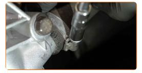
Install the water pump pulley.
