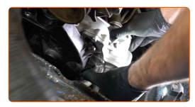
Tighten the water pump fasteners. Use a combination spanner #13. Use a drive socket #13. Use a torque wrench. Tighten it to 14 nm torque.
