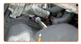
Remove the thermostat housing.
