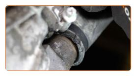
Drain the coolant from the engine.
