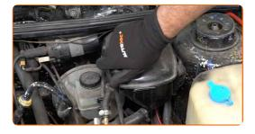
Remove the fender protection cover.
