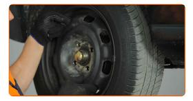
Remove the hub bearing protection cap. Use a flat metal-working chisel. Use a hammer. Use a flat screwdriver.
