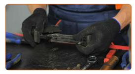
Perform further demounting of the upper retaining spring and the adjuster mechanism. Use pliers.
