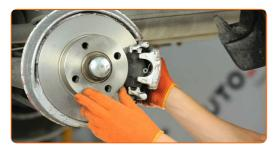
Use a combination spanner #15. Use a combination spanner #13. Use a torque wrench. Tighten it to 35 Nm torque.
