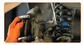
Remove the caliper bracket.
