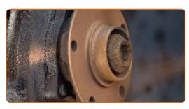
17 Install the brake disc.
