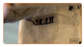
11 Remove the brake caliper.
