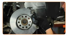
27.1 Install the brake caliper and fix it.
