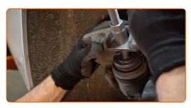
14 Remove the brake pads.
