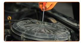
Release the air filter cover clips.
