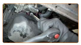
Remove the thermostat housing.
