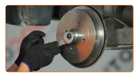
10 Remove the brake drum.
