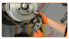
17.1 Install the brake caliper and fix it.
