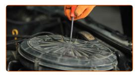
Release the air filter cover clips.
