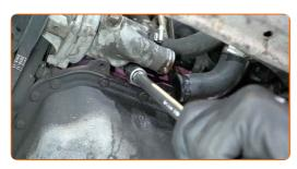
Remove the thermostat housing.
