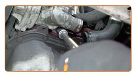
9 Remove the thermostat housing.
