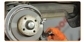
15 Remove the brake disc.
