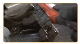
19 Install the brake caliper bracket.
