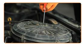
Release the air filter cover clips.
