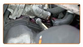
Remove the thermostat housing.
