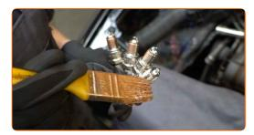
Install the new spark plugs into their mounting seats. Use the spark plug socket #21.
