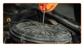
Release the air filter cover clips.
