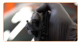
Remove the blade from the wiper arm.
