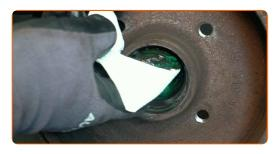
Remove the inner race of the wheel bearing from the brake drum. Use 3-Arm Gear Puller. Use a bush and bearing driver set.
