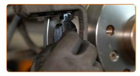
Install the brake caliper and fix it. Use a combination spanner #17. Use a drive socket #13. Use a ratchet wrench.
