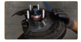
28 Install the hub bearing together with the brake disc protection plate.
