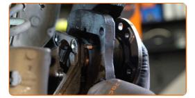
Tighten the fastener of the wheel hub bearing. Use a drive socket #16. Use a torque wrench. Tighten it to 50 Nm torque.+45°
