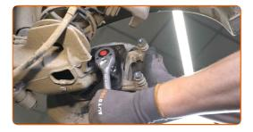
16 Remove the caliper bracket.
