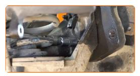
Remove the hub bearing together with the brake disc protection plate.
