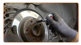
19 Remove the brake disc. Use a hammer.
