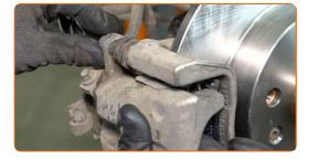
Tighten the brake hose fastener. Use a drive socket #E11. Use a torque wrench. Tighten it to 15 Nm torque.
