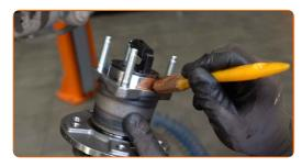
Install a new wheel hub bearing.
