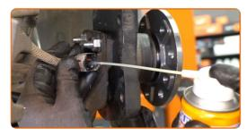
Attach the ABS sensor connector.
