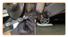
9 Remove the fastening bolt.
