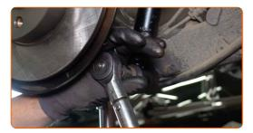
Tighten the top shock absorber fastening. Use a drive socket #E18. Use a torque wrench. Tighten it to 90 Nm torque.
