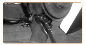
Remove the mounting from under the rear axle beam.
