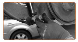
Tighten the lower fastener of the shock absorber. Use a drive socket #E20. Use a torque wrench. Tighten it to 130 Nm torque.
