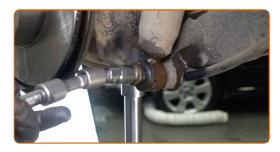
9 Remove the fastening bolt.
