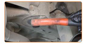
Pull down the rear suspension beam. Use a crowbar.
