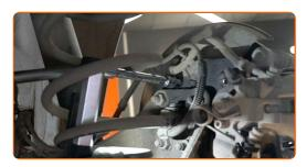
Clean the brake caliper fasteners. Use a wire brush. Use WD-40 spray.
