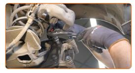
Remove the caliper bracket.
