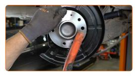
20 Install the brake disc.
