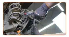
11 Remove the brake caliper. Use a crowbar.
