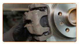
Tighten the brake hose fastener. Use a drive socket #E11. Use a torque wrench. Tighten it to 15 Nm torque.
