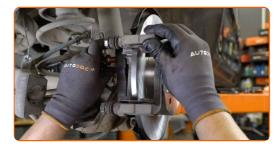
Tighten the brake caliper bracket. Use a drive socket #E16. Use a torque wrench. Tighten it to 100 nm torque.
