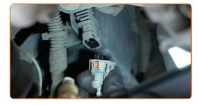
Unscrew the oxygen sensor fastener. Use a flare nut spanner #22.
