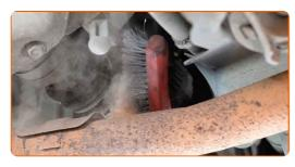
Detach the oxygen sensor connector.
