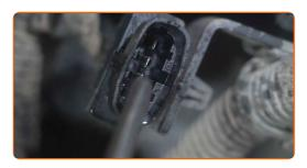
Attach the oxygen sensor connector.
