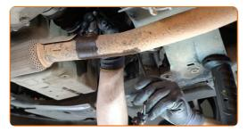
Tighten the oxygen sensor fastener. Use a combination spanner #22. Use a torque wrench. Tighten it to 32 Nm torque.
