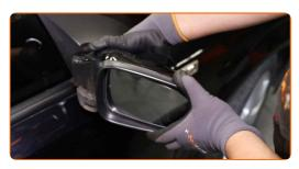
Carefully release the mirror glass from its attachment. Use a plastic trim tool.
