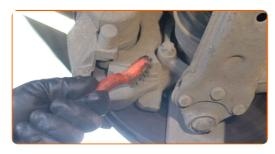
Unscrew the caliper bracket fastening. Use a drive socket #18. Use a tap wrench.
