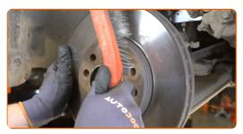
Unscrew the brake disc fastening. Use Torx T30. Use a ratchet wrench.
