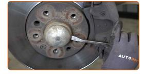
Loosen and remove the hub nut. Use a drive socket #32. Use a tap wrench.
