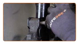
Tighten the hub. Use a drive socket #E18. Use a torque wrench. Tighten it to 90 Nm torque.+45°
