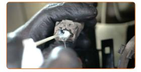
Attach the ABS sensor connector.
