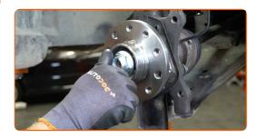
Apply some copper grease to the hub where it contacts the brake disk.
