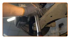
Tighten the wheel hub nut. Use a drive socket #32. Use a torque wrench. Tighten it to 250 Nm torque.
