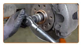
Install the cap of the hub nut.
