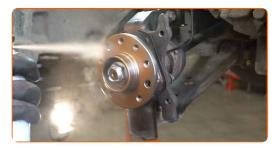
41 Install the brake disc.
