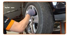
Remove the wheel hub nut cap. Use a hammer. Use a crowbar.
