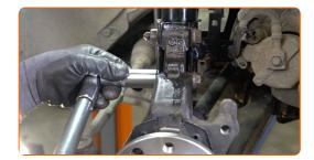
Treat the ABS sensor connector. Use dielectric grease.
