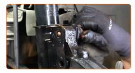
Tighten the lower fasteners connecting the shock strut to the steering knuckle. Use a combination spanner #18. Use a drive socket #18. Use a torque wrench. Tighten it to 120 Nm torque.
