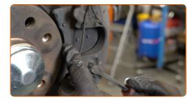
11 Remove the brake caliper.
