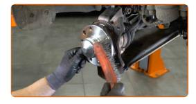
20 Install the brake disc.
