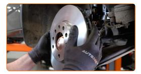
Tighten the brake disc fastening. Use Torx T30. Use a torque wrench. Tighten it to 7 nm torque.
