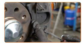
11 Remove the brake caliper.
