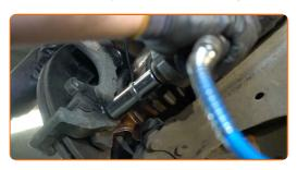
Remove the caliper bracket.
