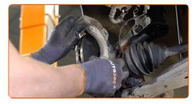
Tighten the brake caliper bracket. Use a drive socket #18. Use a torque wrench. Tighten it to 100 nm torque.
