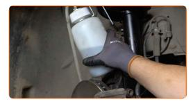
Tighten the brake caliper bleed screw. Use a combination spanner #9. Use a torque wrench. Tighten it to 5 Nm torque.
