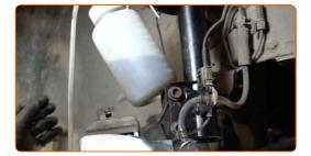
Bleed the brake caliper system. Without starting the engine, press the brake pedal several times until you feel significant resistance.
