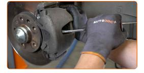
Clamp the brake hose off using a brake hose clamp.
