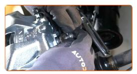
Tighten the fastener connecting the brake pipe to the brake caliper. Use a drive socket #11. Use a torque wrench. Tighten it to 30 Nm torque.
