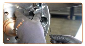
Remove the brake hose clamp.
