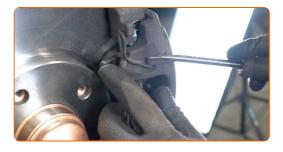
Remove the brake caliper.
