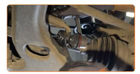
Tighten the fastener connecting the stabilizer link to the shock strut. Use a combination spanner #18. Use a drive socket #18. Use HEX No.H5. Use a torque wrench. Tighten it to 55 Nm torque.
