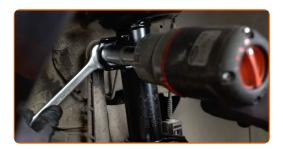
Unscrew the fastener connecting the stabilizer link to the stabilizer bar. Use a combination spanner #18. Use a combination spanner #17.
