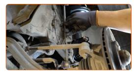
Tighten the stabiliser link fastener. Use a combination spanner #18. Use HEX No.H5.
