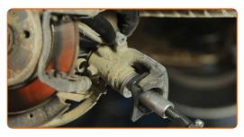
17 Install the brake caliper and fix it.
