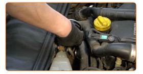
Screw the new filter into its place. Use the 76-14F socket. Use a torque wrench. Tighten it to 25 Nm torque.
