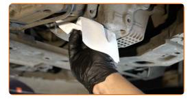
Screw in the new drainage plug and tighten it. Use square oil drain plug socket No.8 Use a torque wrench. Tighten it to 20 nm torque.
