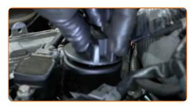
Tighten the oil filler cap.
