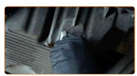
Screw in the new drainage plug and tighten it. Use a drive socket #19. Use a torque wrench. Tighten it to 25 Nm torque.
