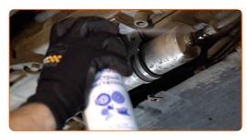
Loosen the fuel filter clamps. Use a flat screwdriver.
