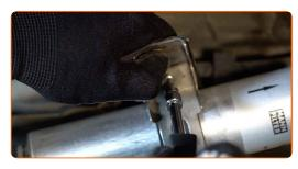
Tighten the fuel filter fasteners. Use a drive socket #13. Use a ratchet wrench.
