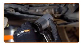
Tighten the fastener of the fuel filter bracket. Use Torx T20. Use a ratchet wrench.
