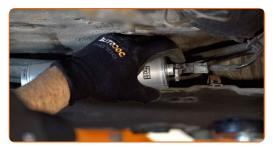
Tighten the fuel supply line fastening. Use a flat screwdriver.
