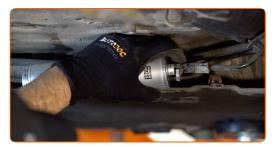
Tighten the fuel supply line fastening. Use a flat screwdriver.
