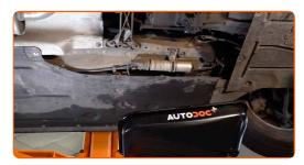
Treat the fasteners attaching the tubes to the fuel filter. Use all-purpose cleaning spray.
