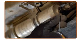
Remove the snap ring of the fuel pressure regulator retainer clip.
