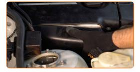
Secure the fastener of the air intake duct. Use HEX No.H5. Use a ratchet wrench.
