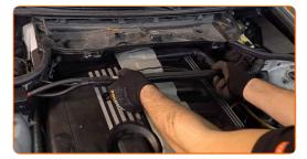
9 Remove the cabin air filter housing.
