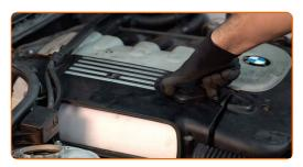
Screw in the fastening screws of the air filter cover. Use HEX No.H5. Use a ratchet wrench.
