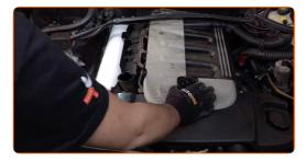
Reinstall the air filter housing.
