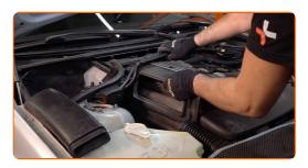
15 Tighten the oil filler cap.
