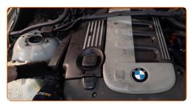
Undo the fastening screws of the air filter cover. Use HEX No.H5. Use a ratchet wrench.
