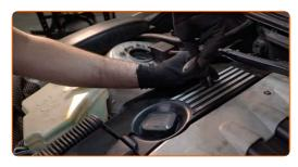
23 Install the air duct housing.
