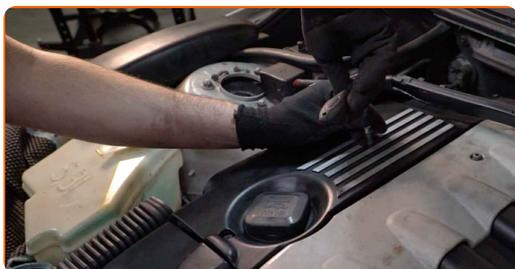
**23** Install the air duct housing.
