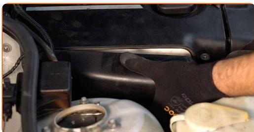
**24** Secure the fastener of the air intake duct. Use HEX No.H5. Use a ratchet wrench.
