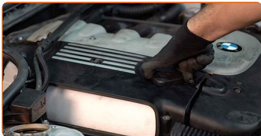
**22** Screw in the fastening screws of the air filter cover. Use HEX No.H5. Use a ratchet wrench.
