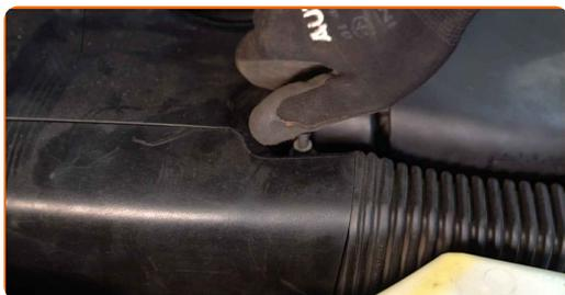
**11** Detach the air duct housing from the air filter housing.
