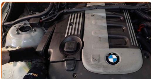
**12** Undo the fastening screws of the air filter cover. Use HEX No.H5. Use a ratchet wrench.
