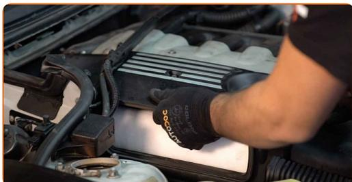
**21** Tighten the oil filler cap.
