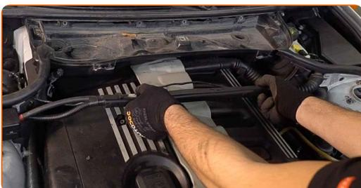
**9** Remove the cabin air filter housing.
