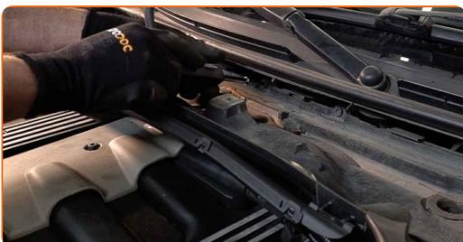
**8** Disconnect the wiring harness from the cabin filter housing.
