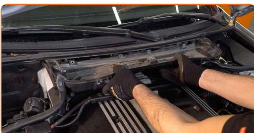
**10** Loosen the air intake fastening. Use HEX No.H5. Use a ratchet wrench.
