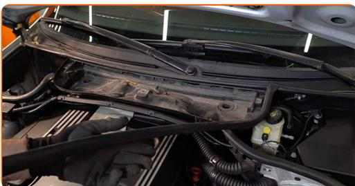
**7** Unscrew the filter housing fastening bolts. Use Torx T20. Use a ratchet wrench.
