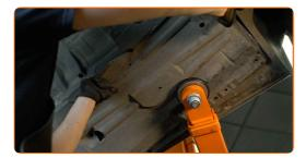
Screw in the fasteners of the underbody cover panel. Use a drive socket #8. Use a drive socket #10. Use a ratchet wrench.
