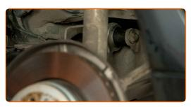
Screw the front arm fastener. Use a combination spanner #18 (2 pieces).
