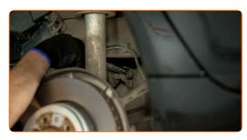
Remove the front fastener of the control arm. Use a crowbar. Use a flat screwdriver.
