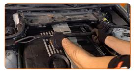
9 Remove the cabin air filter housing.
