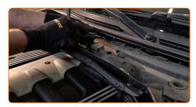
Disconnect the wiring harness from the cabin filter housing.
