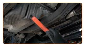
Unscrew the drain plug. Use a drive socket #19. Use a tap wrench.
