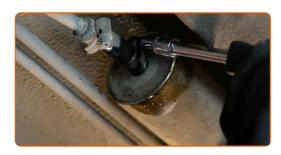
Disconnect the fuel supply lines from the fuel filter.
